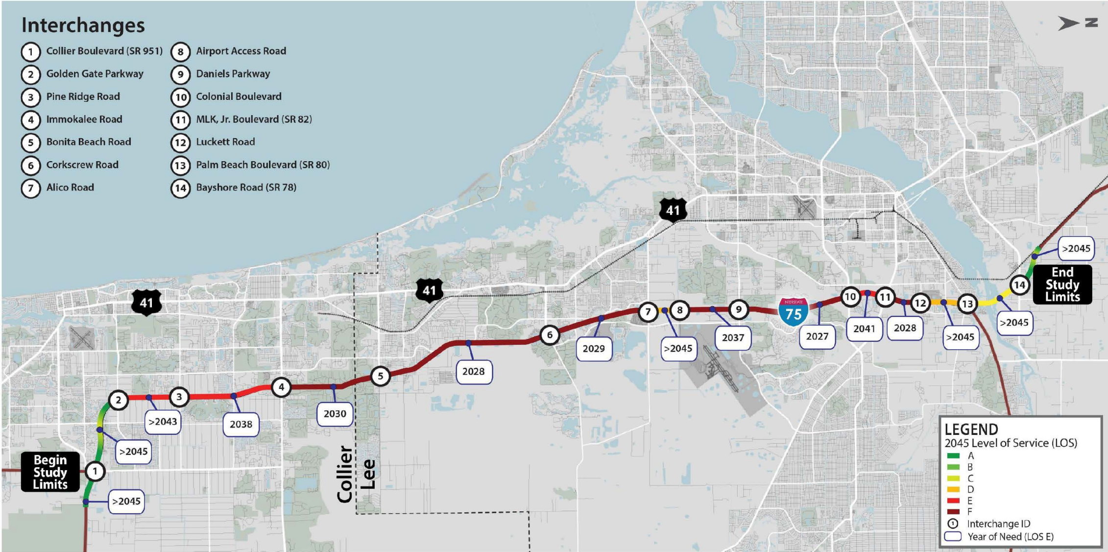
Figure 5-6: No Build Design Year (2045) Southbound I-75 Mainline Years of Need and Level of Service
