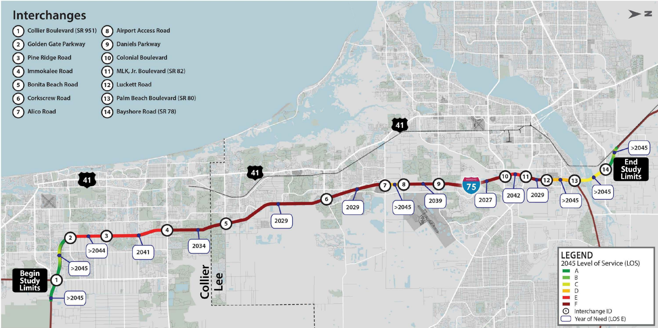
Figure 5-5: No Build Design Year (2045) Northbound I-75 Mainline Years of Need and Level of Service
