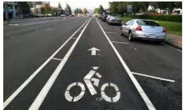
Figure 29. Buffered Bicycle Lane
