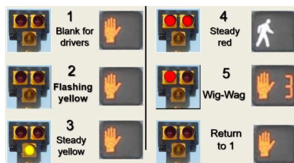
Figure 3-19: Pedestrian Hybrid Beacon Sequence
