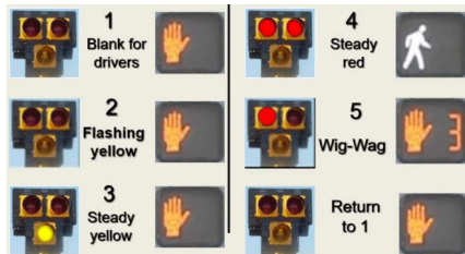
Figure 3-19: Pedestrian Hybrid Beacon Sequence
