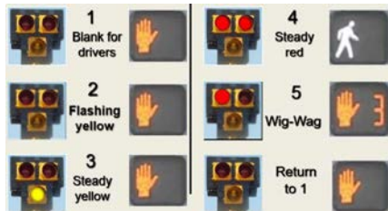
Figure 3-19: Pedestrian Hybrid Beacon Sequence
