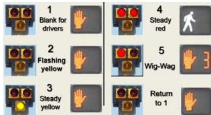
Figure 3-19: Pedestrian Hybrid Beacon Sequence
