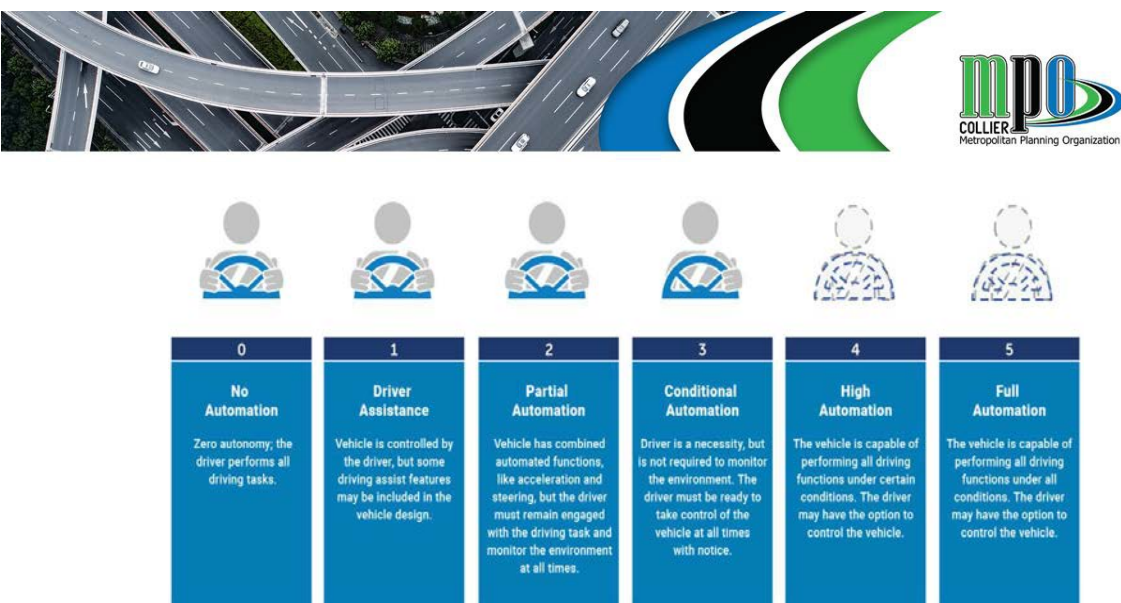
Figure 3-23: Vehicle Autonomy Levels and Features
