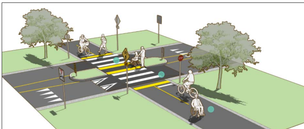
Figure 41. Shared Use Path Crossing
