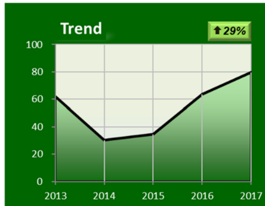
Figure 18. Veh Miles Between Road Calls (000's)
